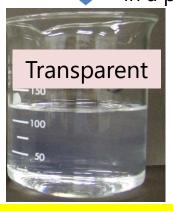
Premix PG enables YT-Lipidure®-PMB to dissolve in EtOH/water mixed solvent without white turbidness.
